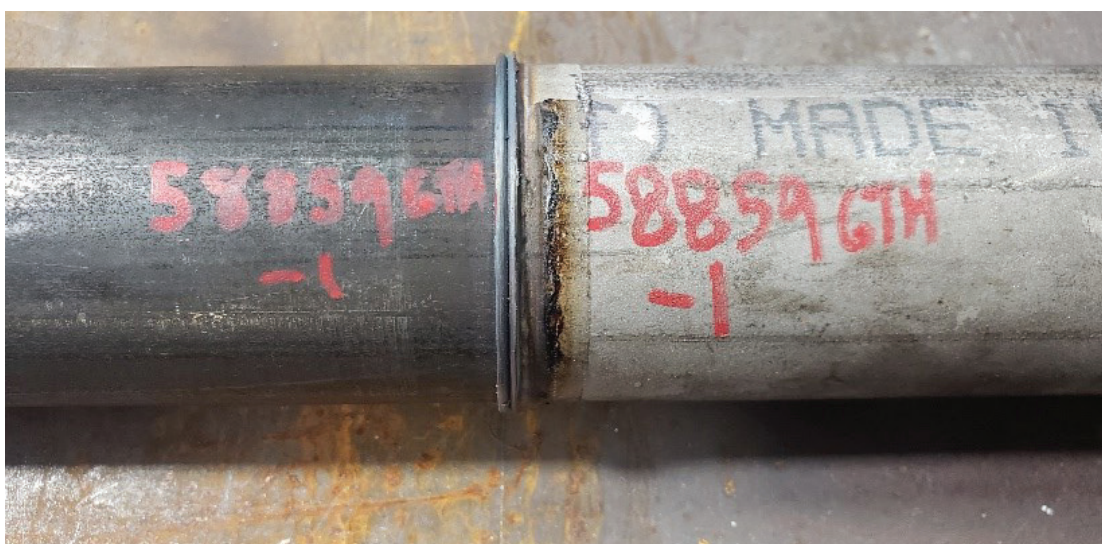
Rotary friction welded T91 to 304H tube.
