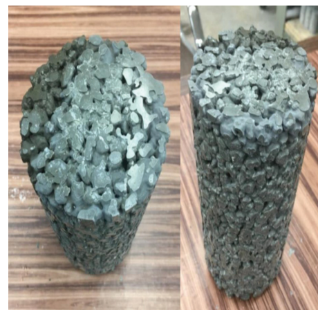
PC specimen prepared with single-sized #4 river gravel aggregate.
