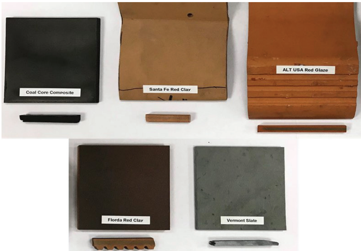
Cut samples of the tile materials tested.
