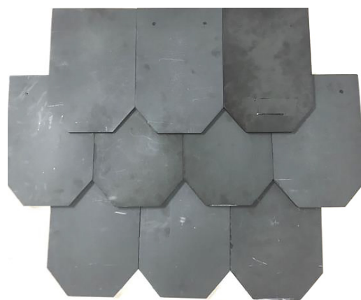
Set of 10 coal-based ceramic roof tiles containing 70% coal.
