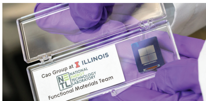
A memristor computer memory chip that contains a coal-derived carbon nanomaterial.
