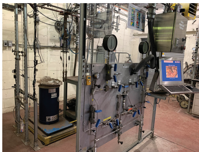
Example of micro-autoclave rig for coal reactivity and liquefaction severity testing.
