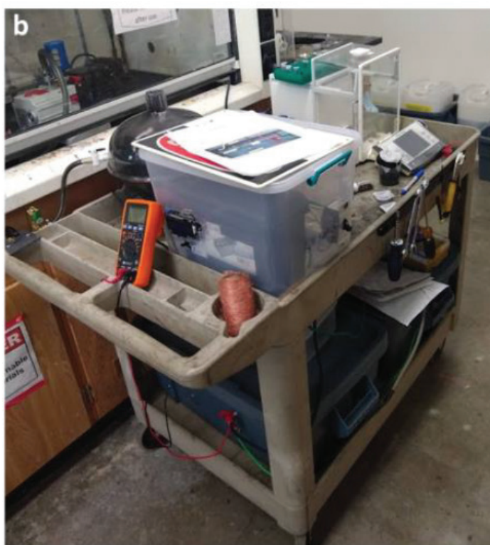
a) Circuit diagram of the FJH station. b) Image of the system on a cart.
