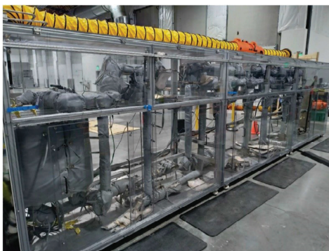
Supercritical CO 2 test loop for generating coal pyrolysis tar.
