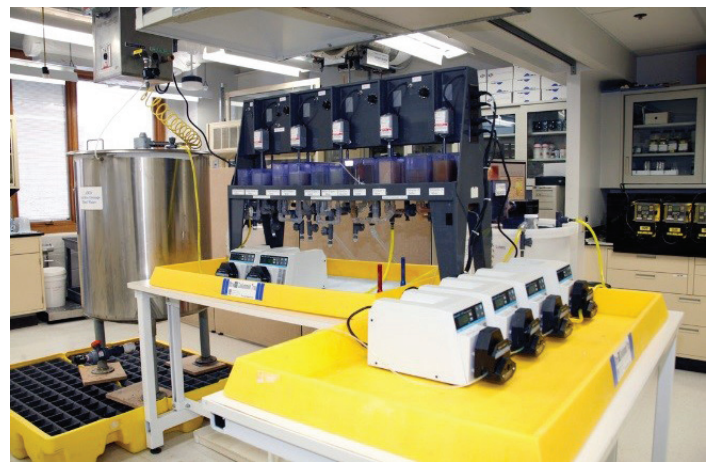
Solvent extraction upgrading of coal ash pregnant leach solutions.
