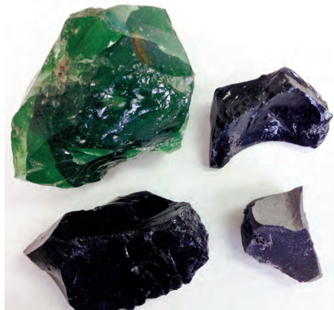
Slag captured from the gasification process (photo provided by Westinghouse Plasma Corp., a division of Alter NRG)
