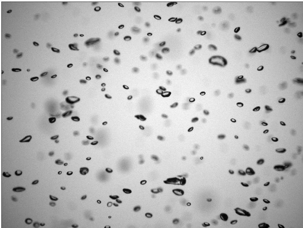
Figure 71: CCD video camera image of an airstone bubble plume at 3.0 NI/min gas flow rate at 11.45 m above the source.
