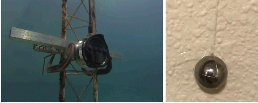
Figure 29: Photographs of (a) The mounted M3 sonar on the underwater tower. (b) The Tungsten Carbide ball used for calibration.
