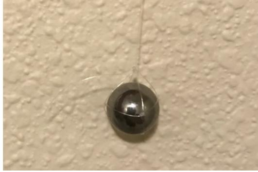
Figure 67: Tungsten carbide calibration sphere.
