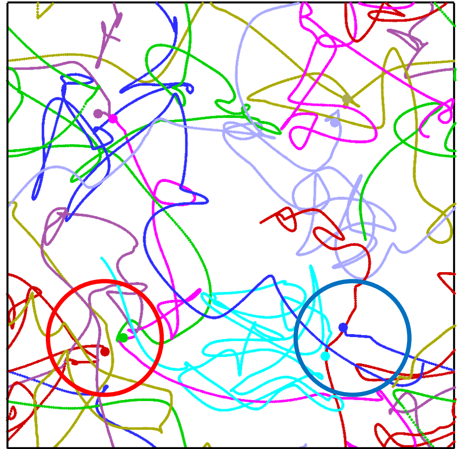
The trajectories of the centroids of spheres in a periodic domain viewed from above. The circles denote the initial conditions. Trajectories leave and enter the domain
