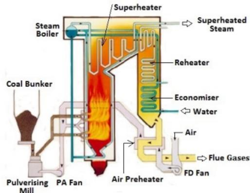
Pulverized coal-fired boiler in thermal-power-plants.
