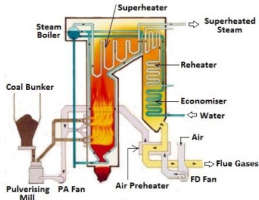
Pulverized coal-fired boiler in thermal-power-plants.
