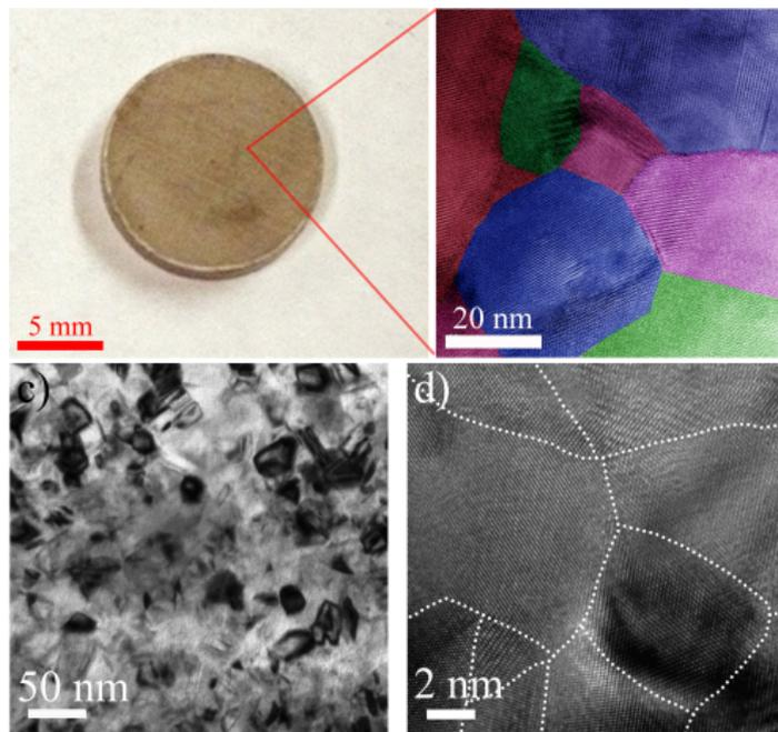
Nanostructured thermoelectric materials.
