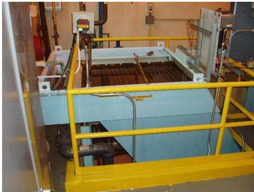
Photo 3.2.6: Pittsburgh Plate Separator.
