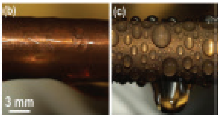
Film-wise vs. drop-wise condensation.
