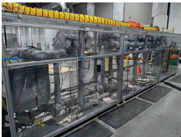
Supercritical CO 2 test loop for generating coal pyrolysis tar.
