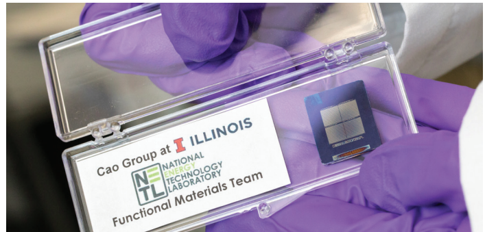
A memristor computer memory chip that contains a coal-derived carbon nanomaterial.
