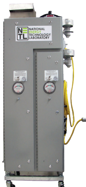
Raman gas analyzer field prototype.
