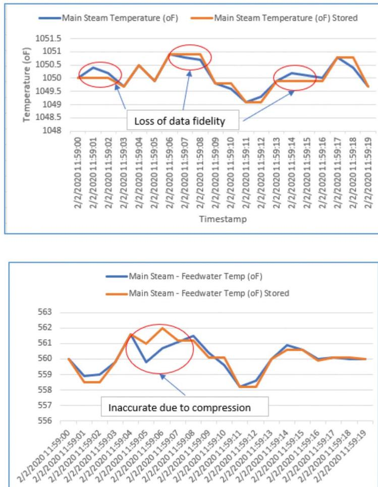
**FIGURE 11.** Main Steam Temperature Data Compression (Left); Main Steam Temperature minus Final Feedwater Temperature (Right) (Original graphs created by author for this report.)
