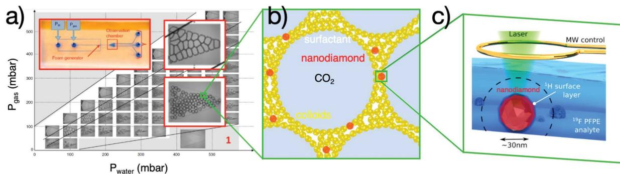
**FIGURE 4.** Generation and analysis of foams for subsurface operations. (a) Foam structure regimes as a function of gas and fluid injection pressure can be visualized in a microfluidic device<sup>[68]</sup>. (b) Pickering emulsions are foams with stability enhanced by colloidal particles in the interfacial phase<sup>[69]</sup>. (c) The components of foam lamellae and local rheological properties could be monitored in situ using NV<sup>-</sup> centers in nanodiamond<sup>[66]</sup>.
