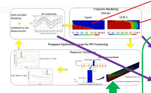
These two pieces of information are combined to obtain *fracture conductivity* distribution in the hydraulic fracture for larger-scale reservoir simulation
