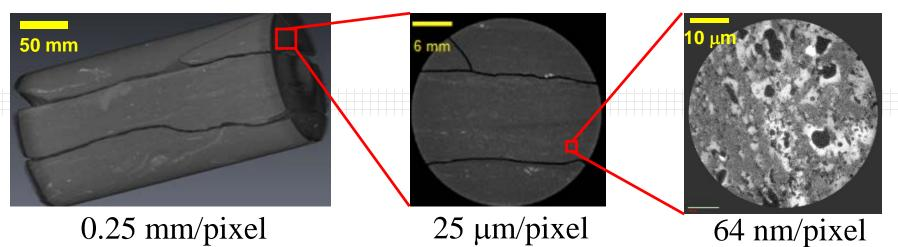
3D, multiscale X-ray CT scanning from core to nm scales.
