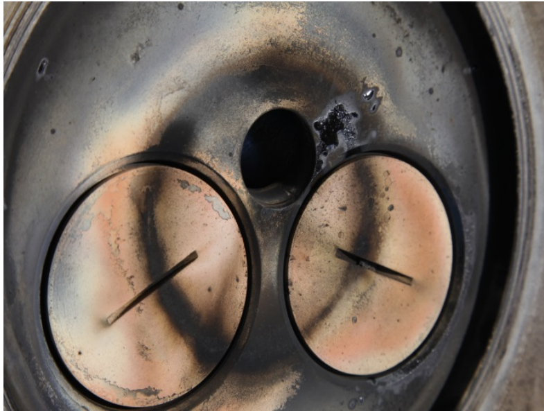
Figure 3-7 Head Valves after 40 hours of Full-Load Operation Using MRC Produced from Yancoal UCC
