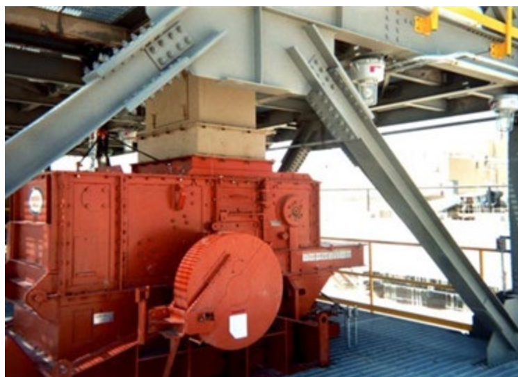
Figure 2-5 Typical Hammer Mill Installation
