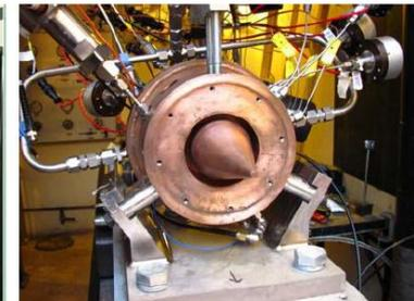
Fig. 3: (a) Schematic diagram illustrating RDE integrated with the mixing chamber, (b) photograph of the high-pressure combustion test rig to be modified for the proposed study, and (c) Example of RDE hardware at Aerojet Rocketdyne that will be utilized in this study.
