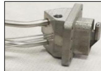
Hot-fire testing with a cobra probe to determine operating limits and hot gas velocity vectors
