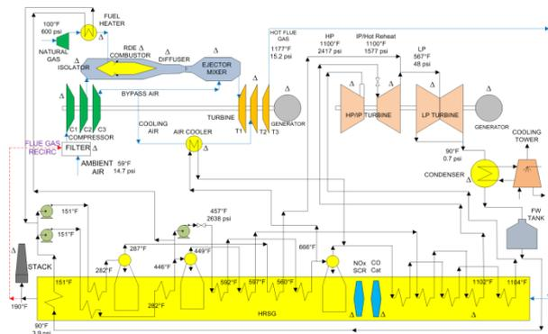
A Natural Gas Combined Cycle system model that has been anchored with RDE test data
