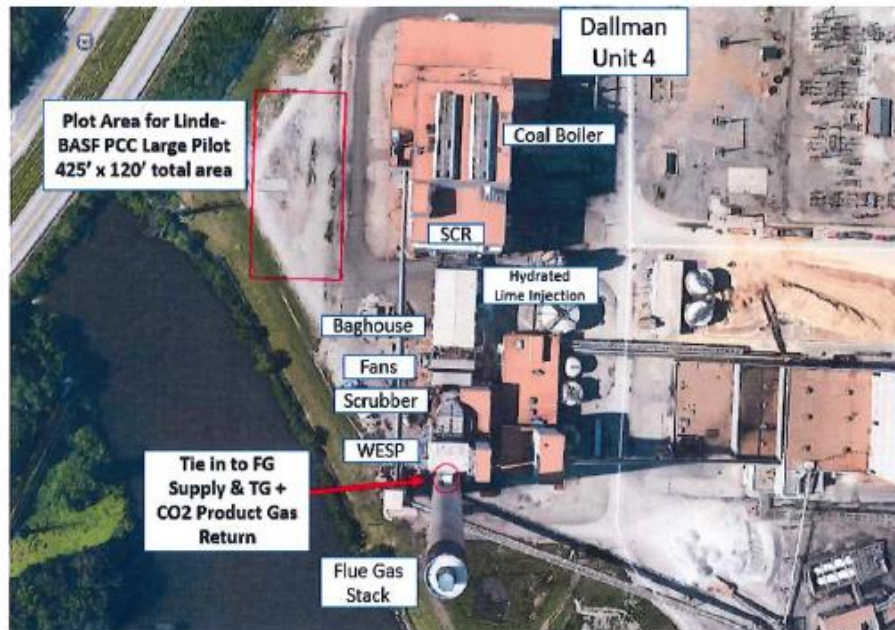
Figure 3 – Location of Pilot Plant on CWLP Facility
