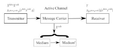
An active network channel uses executable code in the packet to impact the channel controlling the relationship between the transmitted sequence X and the received sequence Y.
