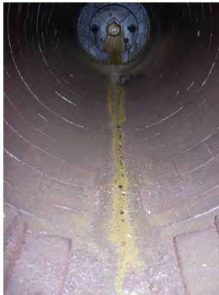
Figure 6. Slag Residue Inside the Combustor
