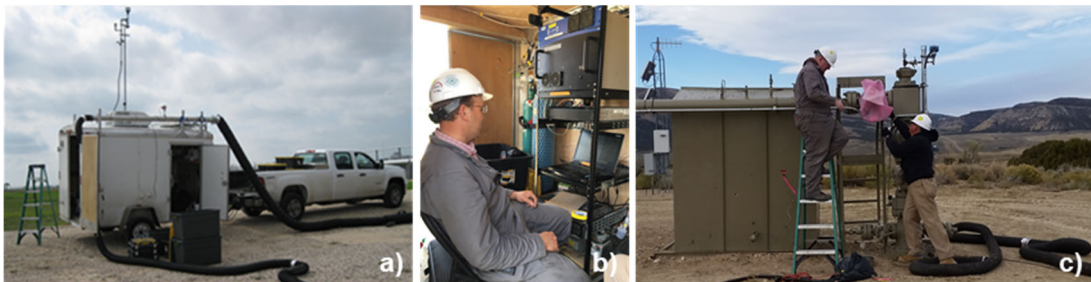
Figure C-2 Photographs of the high flow sampling system in operation: a) entire system, b) interior of the trailer, and c) bagging a valve for sampling.
