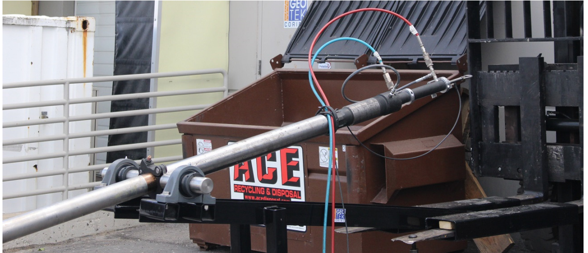
Figure 1, VFFPT Test Fixture mounted to a forklift. Note large bearings and lifting clamp.
