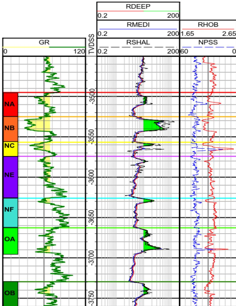
Figure 3. Type log of the Schrader Bluff NB and OA sands.
