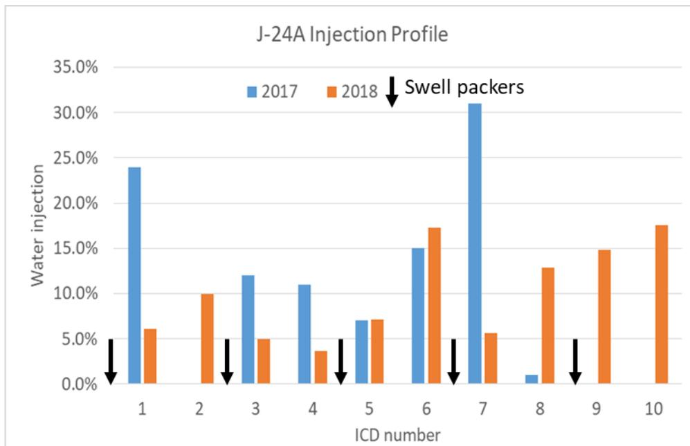
Figure 18. J-24A injection profile log
