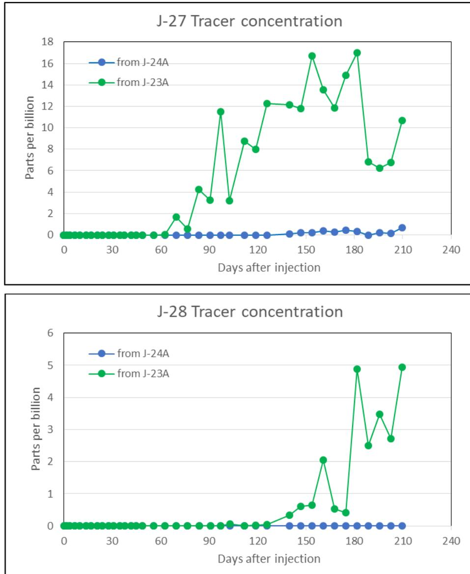
Figure 19. Tracer concentrations in produced water
