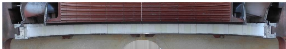
Shroud ~8 cm x 15 cm first stage shroud 96 per full set – 160 MW machine
