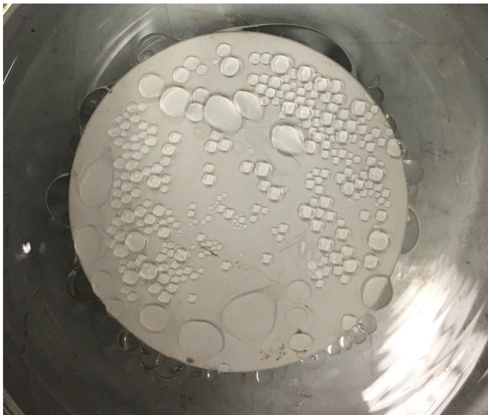
Figure III.2.19: Oil spontaneously effusing from the ceramic as water is imbibed.
