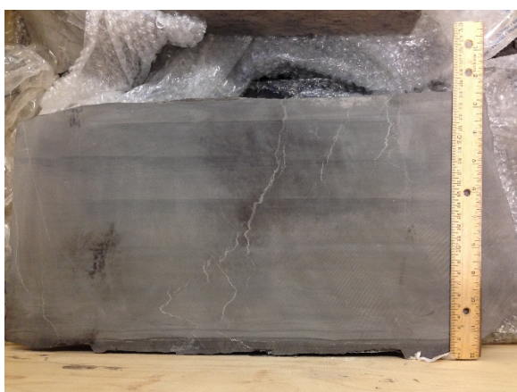
Figure III.2.2: Photos of half-meter scale Niobrara shale block. Left-broken on bedding plane, right-saw cut.
