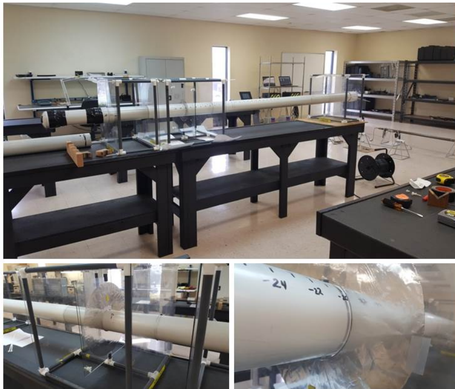
Figure 4.8: Laboratory experimental setup: an outer shell backbone (horizontal pipe) containing coils, fracture model inside a holder (middle box), and two outer shell backbone holders (left and right boxes).
