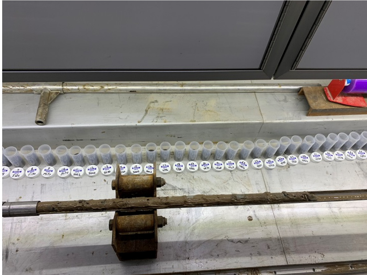
Core barrel containing continuous side-wall cores
