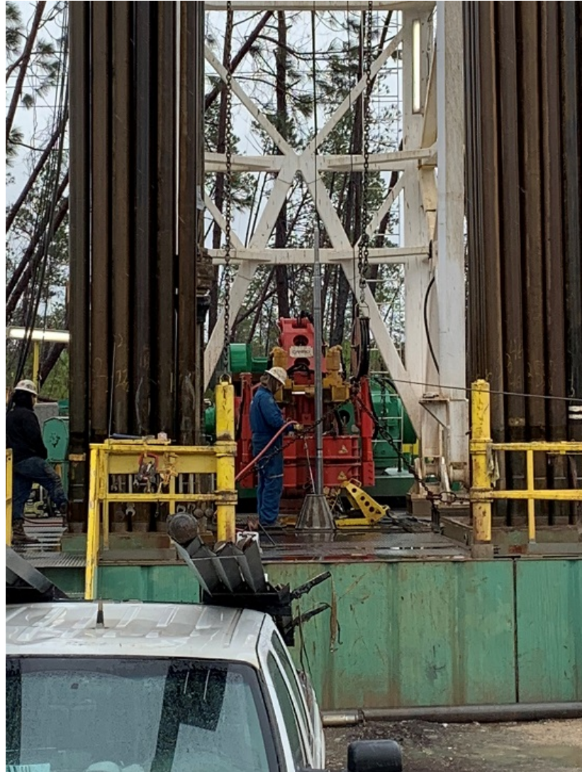
Retrieving the core barrel via wireline
