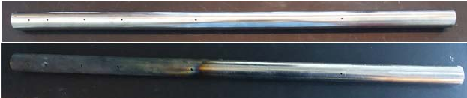
Inconel WG before and after testing at 1,200° C
