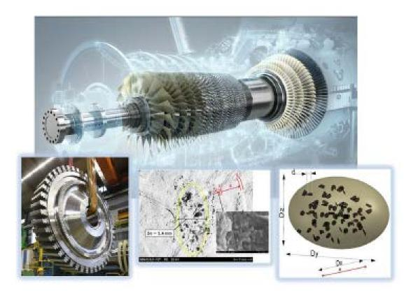
Understand crack nucleation and growth from forging flaws to enable higher temperature, higher load operation
