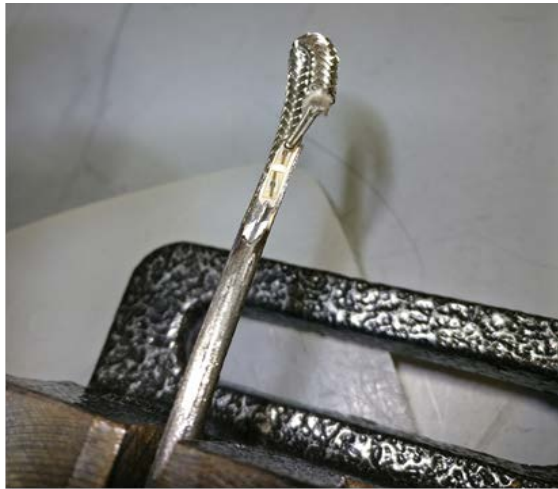
SAW sensor mounted prior to insertion in probe
