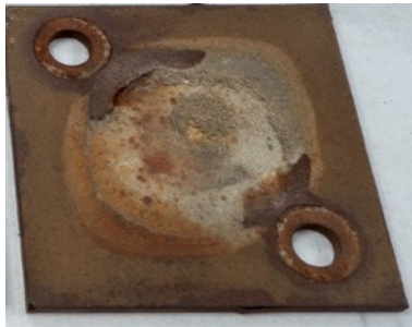
Corrosion of untreated carbon steel coupon
