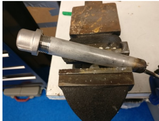
SAW sensor inserted in high-temperature 6" probe
