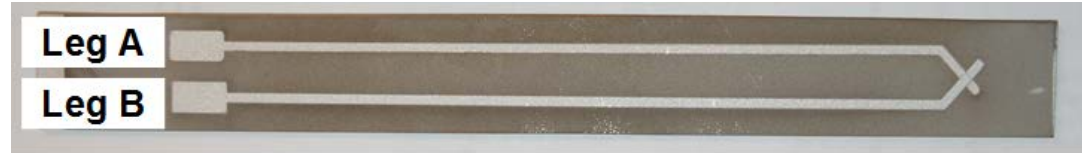
Thermocouple deposited on a performance and calibration test bar.
