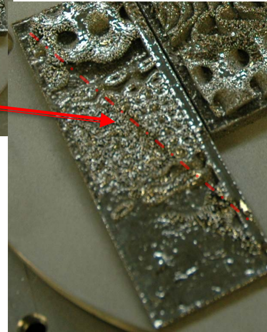
Stress fracture in part
