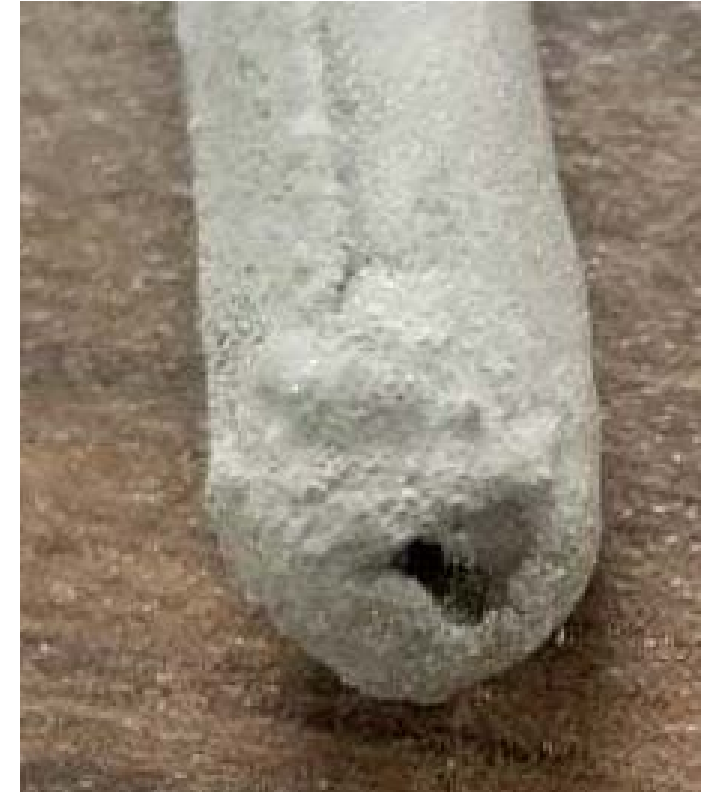
Damaged tip of thermocouple
