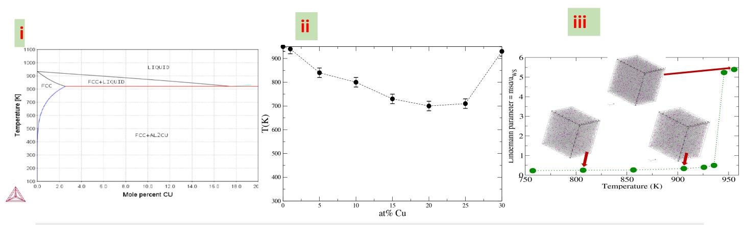
i phase-diagram of AlCu from Calphad calculations ii Liquidus part of the AlCu phase-diagram computed from MD, corresponding to T values of zero velocity of solid-liquid interface
