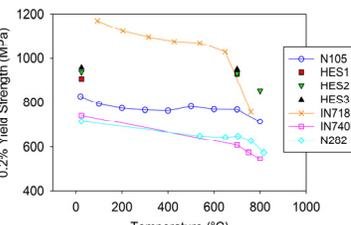
NETL applied HEA principles to re-design the matrix of gamma prime precipitation strengthened Ni-superalloys. The NETL High Entropy Superalloys (HEA) have good elevated temperature strength compared to conventional alloys used in advanced fossil energy power systems. Evaluation of the performance is continuing.
