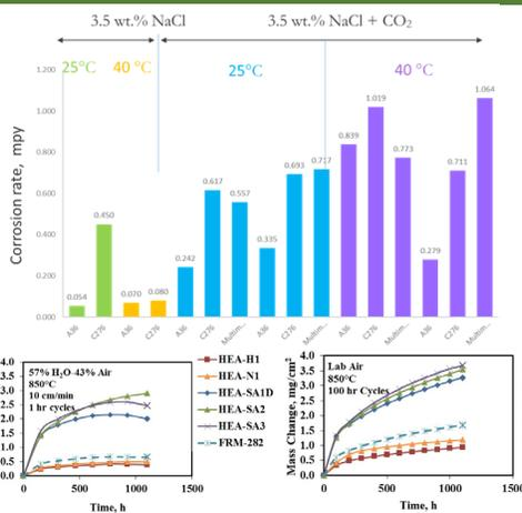
The high temperature oxidation behavior of a FeNiCoCrMn single phase austenitic HEA. Test was done at 750 (not shown) and 850°C. The oxidation resists of NETL HEA-N1 and HEA-1N compare favorably to the commercial superalloy 282.
