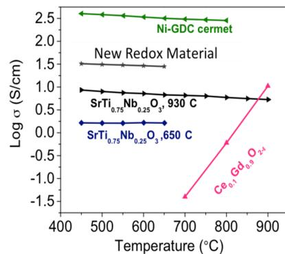
**Redox ceramic anode** → small Δoxygen = small dimensional change (0.4 vol%)
