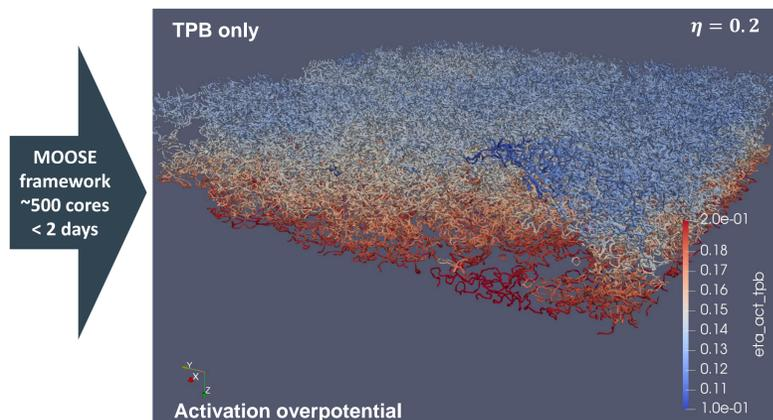
Visualization of a computed variable solution field. In this instance the activation overpotential at the TPBs is visualized in 3D space. Notice that the large boulder affects the surrounding local electrochemistry, located at the top of the boulder.
