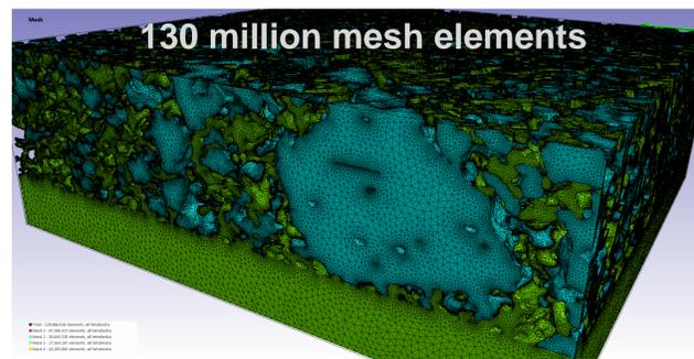
Large-scale meshed microstructure. The size is 30 x 30 x 10 [μm]. The number of mesh elements is 130 millions. The presence of an abnormally large feature is shown in the image.
