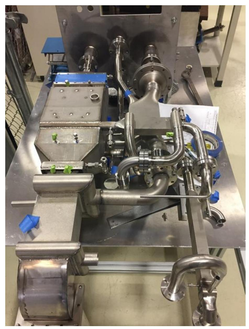
A vacuum insulation box covers the hot BOP components. The box is constructed of a stainless steel shell filled with microporous insulation. Removing air provides excellent insulation performance in a small footprint.
