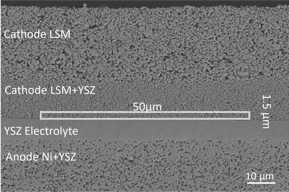
Repeat area scan 30 times across the 5mm cathode/electrolyte interface under Cr source.
