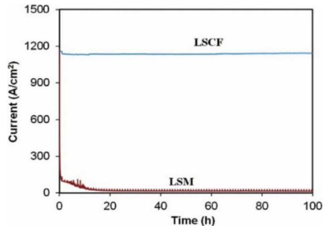
Fig. 2 – I–t curves of LSM/YSZ/Pt and LSCF/GDC/Pt half cells. Tests were conducted at 1023 K with 150 sccm of 3% H<sub>2</sub>O/air flowing through a Cr<sub>2</sub>O<sub>3</sub> powder bed and an applied bias of 0.5 V.
