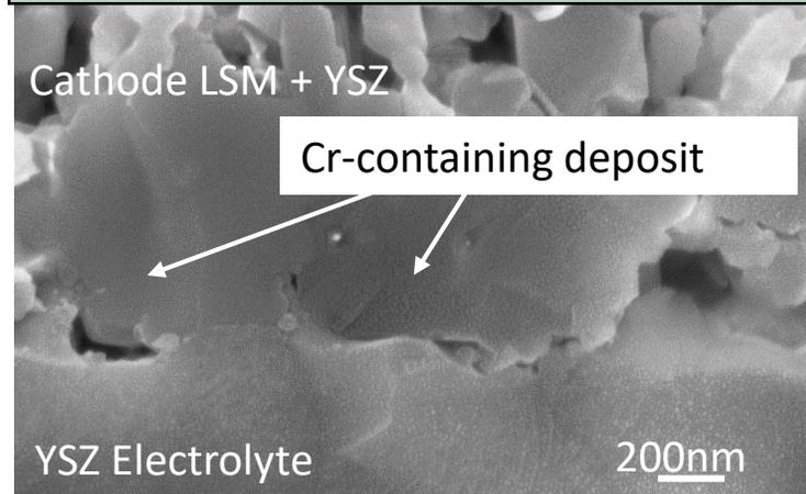
Large Cr-containing particles at cathode/electrolyte interface.
