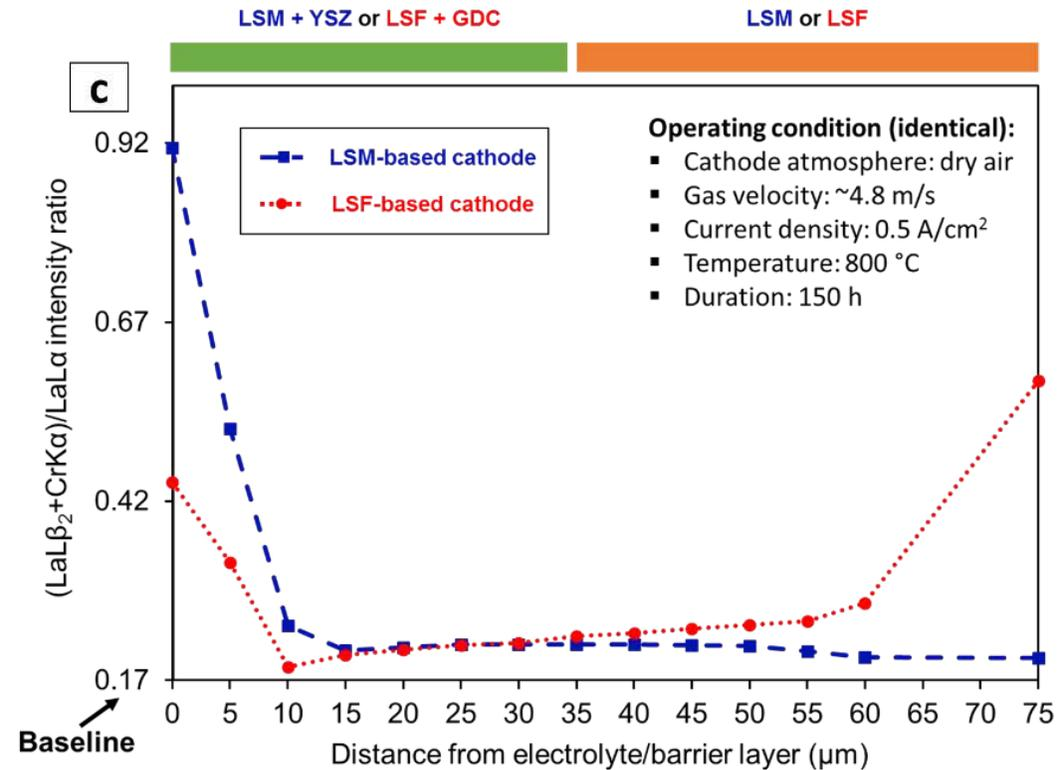
LSF cathodes are more tolerant to chromium poisoning than LSM cathodes
