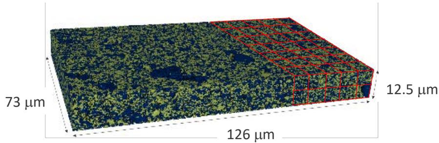
3D Reconstruction of SOFC Electrodes
