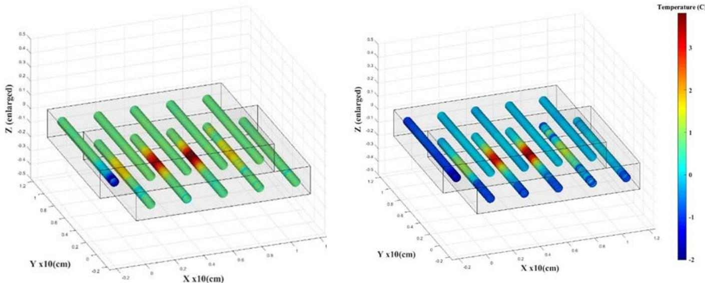
Thermal transients at 30 and 90 s from 5×5 cm<sup>2</sup> ASC at 750°C with H<sub>2</sub> fuel after 2A load
