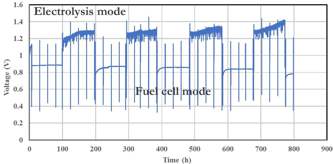
Cell voltage variation under cyclic Fuel Cell/Electrolysis operation for 800 h
