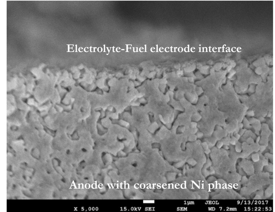
Delamination and Ni phase coarsening are evident from the fuel cell tested under electrolysis mode.
