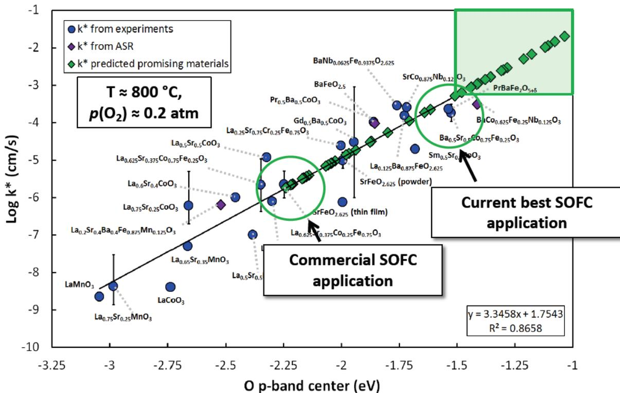
Surface exchange coefficient versus  $O$   $p$ -band center
