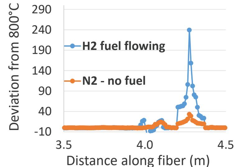
Failure detection: Temperature spike from cracked cell at 800°C
