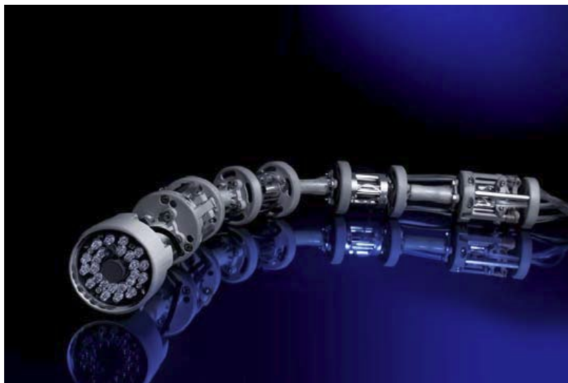
3- and 4-inch pneumatic pipe crawler developed at Florida International University.
