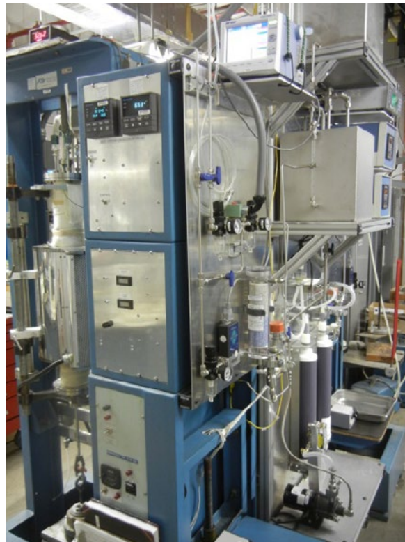
Left: Servo-hydraulic creep-fatigue machine. Right: Thermal cyclic creep machines allowing testing in steam.
