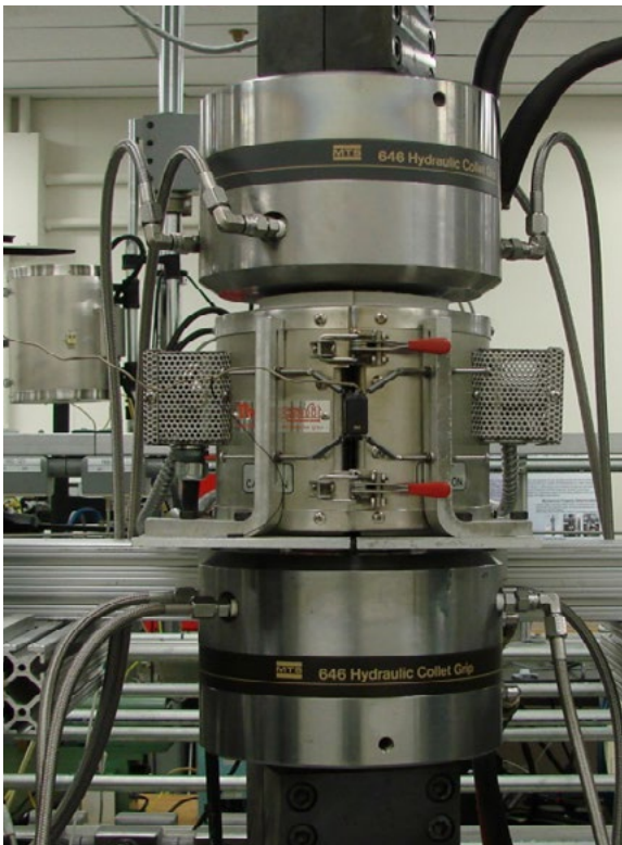
Left: Servo-hydraulic creep-fatigue machine. Right: Thermal cyclic creep machines allowing testing in steam.
