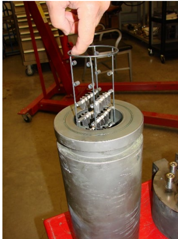
Specimen coupon holder being loaded into ORNL high-pressure autoclave for testing in supercritical carbon dioxide at 750 °C/300 bar.
