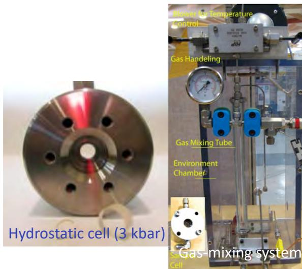
Hydrostatic cell (3 kbar)
