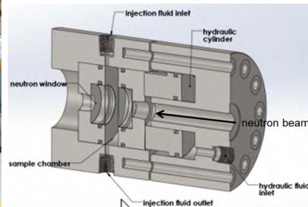
Flow-through compression cell for simulating pore pressure (500 bar) + overburden stress (100 bar).
