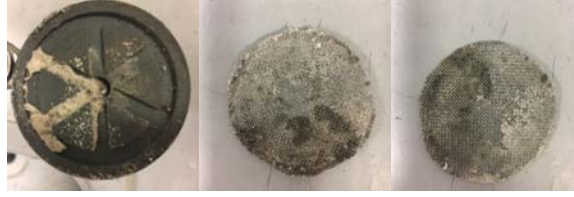
Figure 5.7. Evidence for fine particles migration (end cap).
