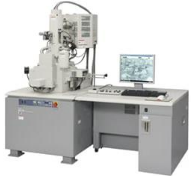
User Facility: Hitachi SU-70 SEM/EDS
