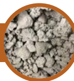
Co-Mingled Steel Slag
