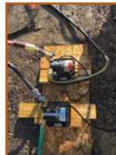
During field testing at the Gorgas power plant (Walker County, AL) solutions are pumped into bailers and inserted into the well.
