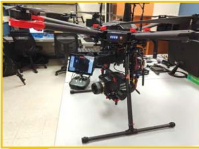
Ronin Gimbal outfitted with an OGI camera; the gimbal allows for controlled omnidirectional pointing of the camera
