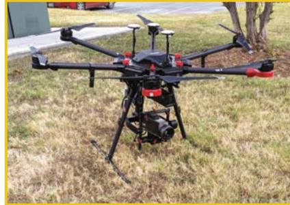
Drone with the optical gas imaging (OGI) camera for data collection.
