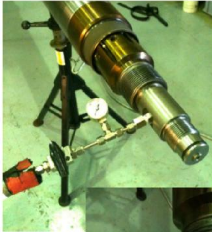
Above: The assembled tool ready for pressure testing.
