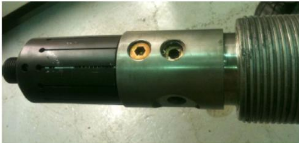
Right: Checking the fit of the HPCT latching 'grabber' (or pulling tool) on the top of the inner tube plug.
