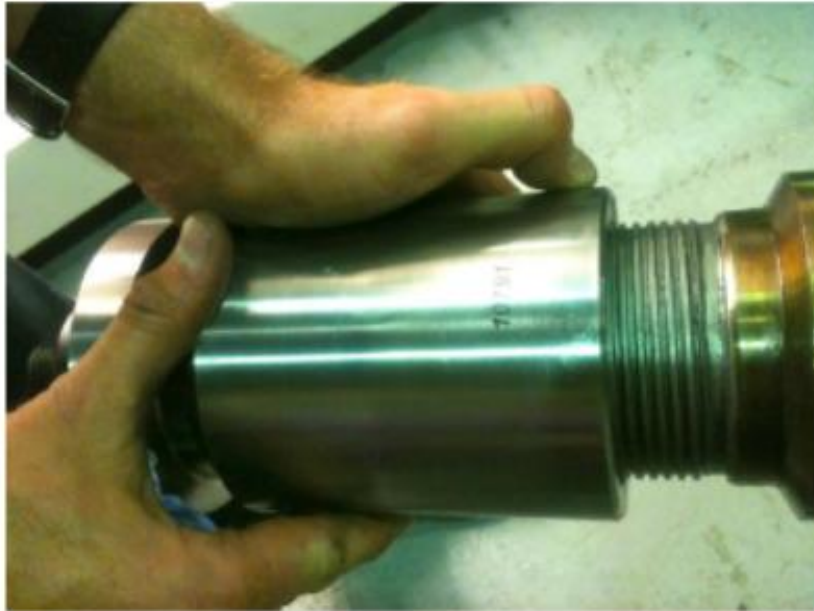
Above: Attaching the connecting flange to the top of the autoclave.
