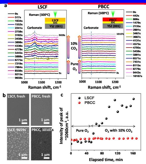
*In situ* Surface enhanced Raman spectroscopic (SERS) study of thin film electrode prepared by PLD. (a) *In situ* SERS spectra of LSCF and PBCC thin film at 500 °C in atmosphere of pure O<sub>2</sub> or O<sub>2</sub> with 10% CO<sub>2</sub>; (b) SEM of fresh films and films after Raman testing in O<sub>2</sub> with 10% CO<sub>2</sub>; (c) Intensity of peak of ~1060cm<sup>-1</sup> observed from thin film LSCF and PBCC surface.
