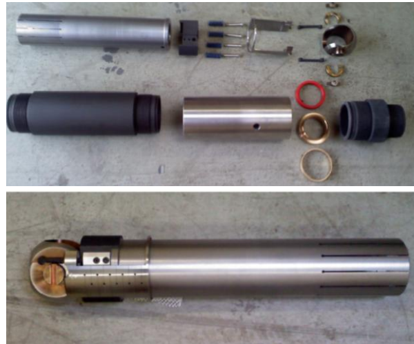
HPTC tool under fabrication. Top panel: ball valve components. Bottom panel: ball valve sub assembly.
