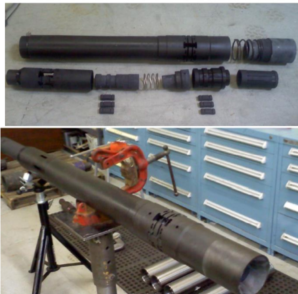
HPTC tool under fabrication. Top panel: latch assembly components. Bottom panel: assembled latch assembly.
