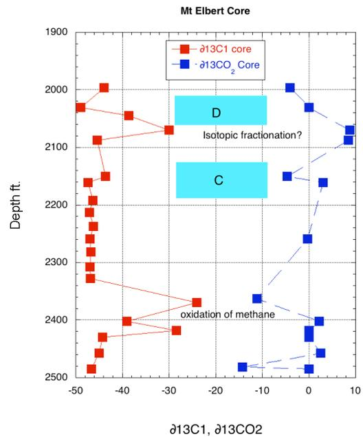
**Figure 6.** Profiles of methane and carbon dioxide isotopic composition with depth of core gas from the Mount Elbert No. 1 well. Light blue bars denote the D and C gas hydrate occurrences. The range of methane isotopic values are similar to the cuttings and flowed gas samples. Post-sampling oxidation of methane may have occurred in the interval of about 2420 to 2350 feet (738 – 717m), while some potential isotopic fractionation maybe occurring at and 2080 to 2050 feet (634 -625m).
