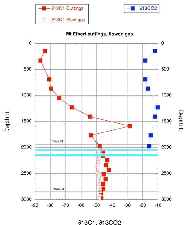
**Figure 4.** Profiles of methane and carbon dioxide isotopic composition with depth of cuttings and flowed gas from the Mount Elbert No. 1 well. Base of permafrost (base PF) and the base of the gas hydrate stability zone (base GH) are given. Light blue lines denote the D and C gas hydrate occurrences.
