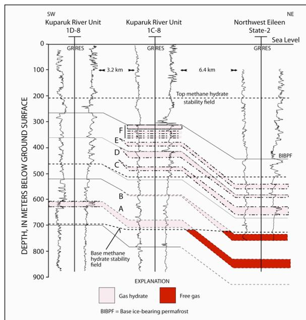
Figure 2. Cross section showing the lateral and vertical extent of gas hydrates and underlying free-gas occurrences in the Prudhoe Bay-Kuparuk River area in northern Alaska. See Figure 3 for location of cross section. The gas-hydrate-bearing units are identified with the reference letters A through F from [2].
