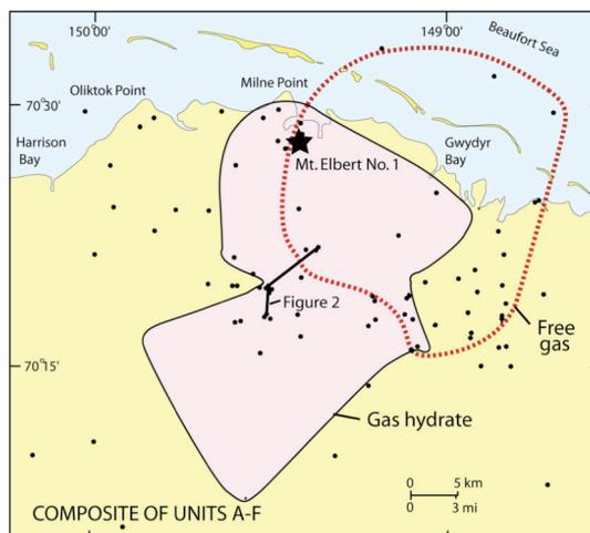
Figure 3. Composite map of the six gas hydrate/free-gas units (Units A-F) from the Prudhoe Bay-Kuparuk River area in northern Alaska. Also shown is the location of the cross section in Figure 2. Dots indicate wells studied in [2]. The Mount Elbert No. 1 well is located north of the cross section in Figure 2, but penetrates an identical stratigraphy.
