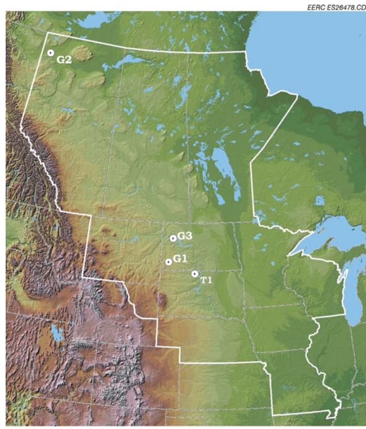
Figure 14. PCOR Partnership Phase II field validation sites (G1 – Lignite coal in North Dakota – CO 2 injected into an unminable lignite coal seam for CO 2 sequestration and possible ECBM production; G2 – Zama, Alberta – Injection site of acid gas for CO 2 sequestration and EOR; G3 – Beaver Lodge, North Dakota – CO 2 injection site for CO 2 sequestration and EOR; and T1 – Wetland sites monitored to establish sequestration potential and MMV technologies).
